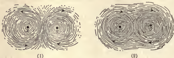
FIG. 336.—Magnetic Fields around Parallel Conductors: (1) When Currents are Flowing in the Opposite Directions; (2) When Flowing in the Same Direction.
